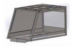
Smooth walls from 4 mm. thickness with suitable reinforcements all around. Front frame with strong beams to stand thrust of hydr.-cylinder for the push-out-plate.
