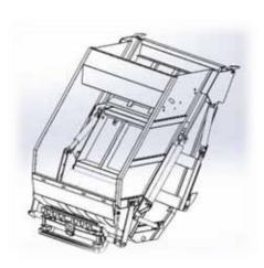
Tailgate connected to body with top hinges. The tailgate structure is consist of 1 sledge, 1 shovel, hopper and their cylinders. When garbage is put inside the hopper, with the help of the sledge and shovel this garbage goes into body and compressed with pushout plate. Sledge moves linearly and shovel moves radially to sweep the garbage inside the body, the sledge runs on sliding rails with roller or shoes.
