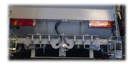
There is a container lifting system powered two double acting cylinder for one 1.1 m³ - 660 lt. standard containers with dome lid opening and tailor design fork type lifting mechanism for containers sized from 0.24 m³ up to 0.30 m³ and skip loader for 6-7 m³ steel container (Design will be approved before order)
