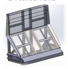
PUSH-OUT plate moves in the NPU rails which are welded above from the floor to the inner sides of the body. Front main plate made from 4 mm. Push-out plate has easily replaceable 8 units of poliamid shoes with bolted connection. Ejection plate moves by means of a double acting telescopic cylinder. It's kept at the rear of the body when it's empty, and moves automatically to the front by means of a counter pressure valve as the refuse is packed in the tailgate.
