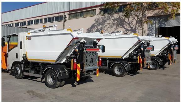
The Minipacker is a rapid and economic solution in collection garbage. İt Provides a modern, Clean and an innovative appearence for the environment. It has a 100% leakage-proof quality and it is much lighter than the other ones since, in this compactor there is no rear cover system present.
